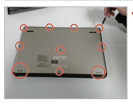
Remove the twelve M2x4mm PH0 Philips head screws.
