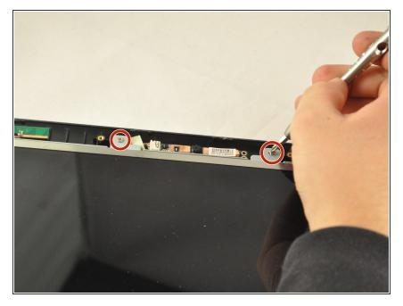
Using the PH1 screwdriver, remove the two .75 cm screws from the top of the screen frame.
