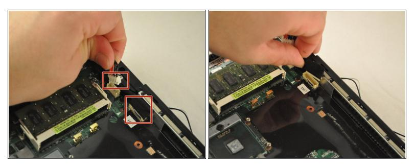
Unplug the wire and black cables on the motherboard, located in the upper-left corner of the laptop.
