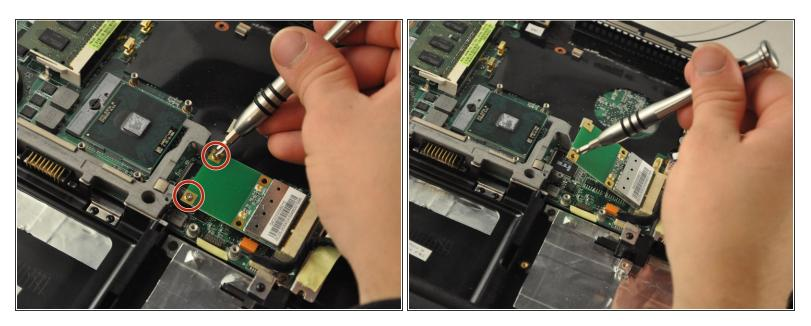
• Using the PH 1 screwdriver, remove the two .25 mm screws from the Wi-Fi card.
