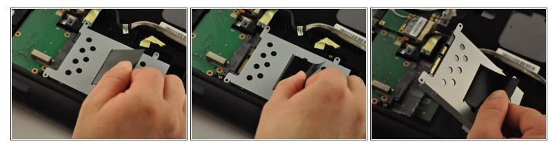
• Pull on the black tab on the driver to slide the driver back, and lift the driver out of the laptop.
