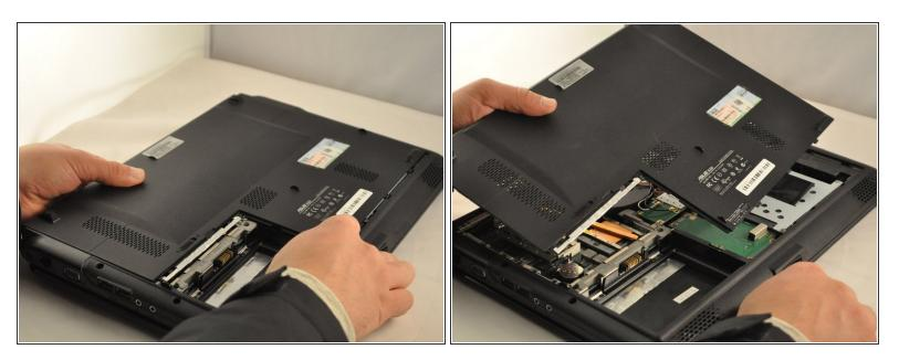
• Remove the bottom panel by sliding it toward the hinges and lifting the back panel up.
