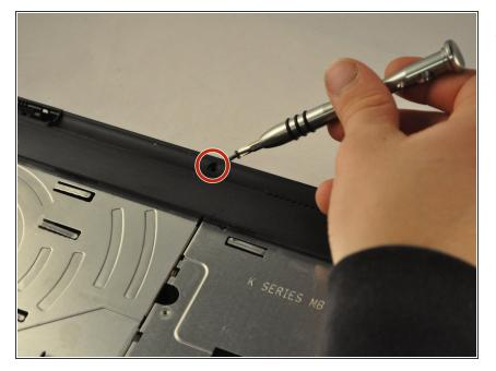
Using the PH1 screwdriver, remove the .75 mm screw from the bottommiddle section was previously covering.
