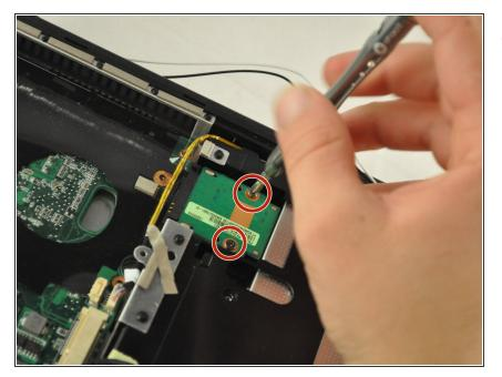
Using the PH 1 screwdriver, remove the two .5 mm screws from the RAM drive.
