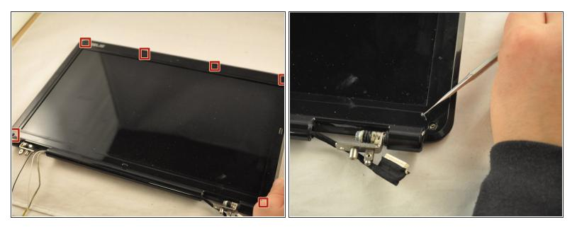
Using a metal spudger, pop off the six rubber screw covers.
