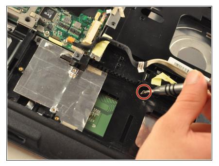
Using the PH1 screwdriver, remove the .75 mm screw from the plastic housing corner, located in the bottom-right corner of the laptop.
