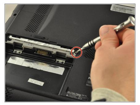
Remove the one .5 mm screw located in the top right corner of the battery compartment.
