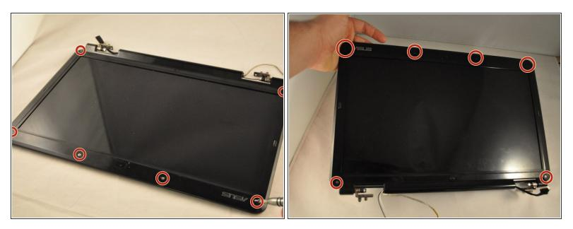
Using the PH1mm screwdriver, remove the six .75 mm screws from the front of the screen frame.
