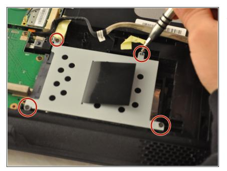
Using the PH1 screwdriver, remove four .75 mm screws from the driver, located in the bottom-right corner of the laptop.
