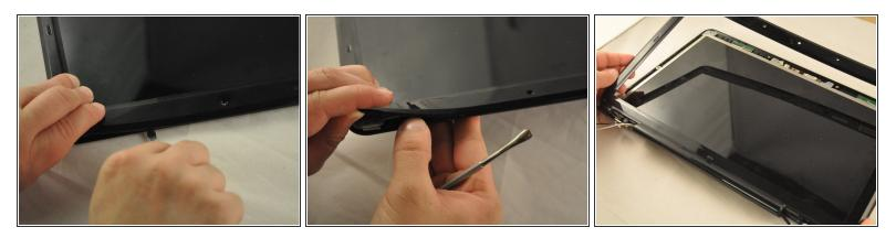
• Use the plastic opening tool or spudger along the edge of the frame, to pry off the frame.
