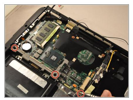
• Using the PH1 screwdriver, remove the three .75 mm screws from the bottom corner of the motherboard.
