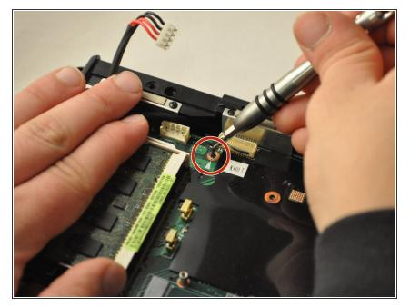
Using the PH 1 screwdriver, remove the .75 cm screw from the topmiddle section of the motherboard.
