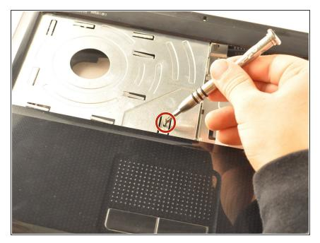
Using the PH 1 screwdriver, remove the .75 cm screw from the bottommiddle section where the keyboard was previously covering.
