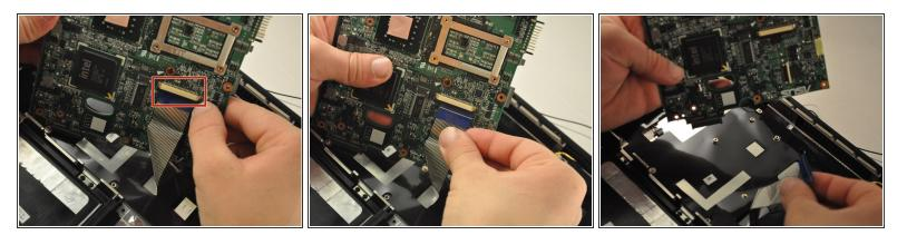
• Gently unplug the ribbon cable from the underside of the motherboard.
