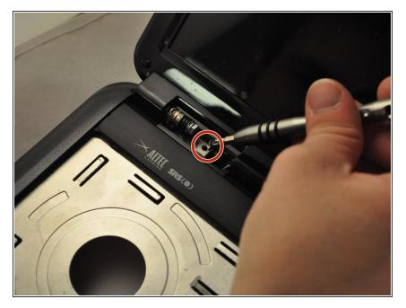
Use the PH1 screwdriver to remove the .75 mm screws from the hinges. Each hinge has one screw.
