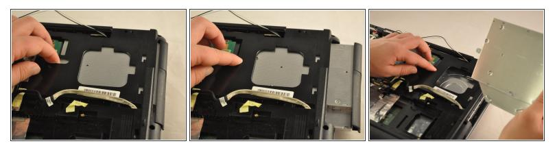
• Slide the disc drive out of its slot.
