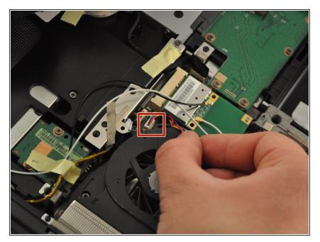
• Unplug the wire cable attached to the fan by pulling it out .
