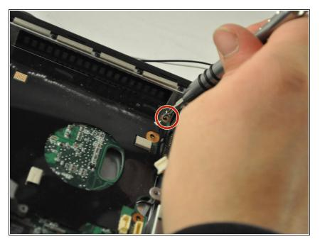
Using the PH1 screwdriver, remove the .75 mm screw from the topmiddle corner of the motherboard.
