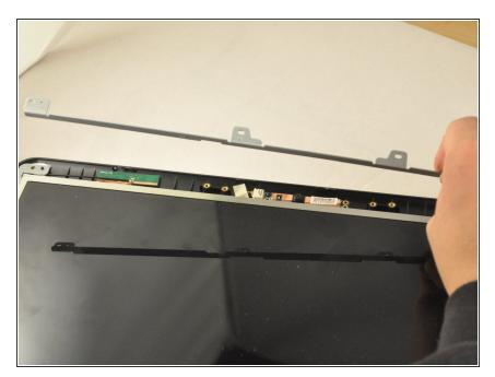
• Lift the bracket off the top of the screen frame.
