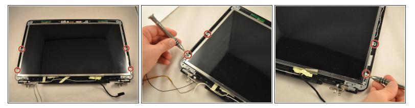
• Using the PH1 screwdriver, remove the four bottom .75 mm screws from the screen frame.
