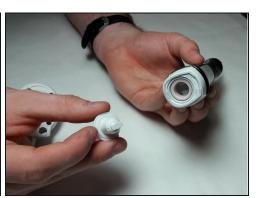
• Use the charging station to remove the a small plastic plug from the end of the toothbrush by inserting the charging station into the end insert and twisting counterclockwise by 90 degrees.
