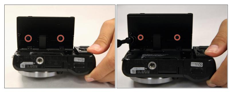
Use a Phillips head 000 screwdriver to remove the two 1.0mm screws on the bigger backplate of the LCD.
