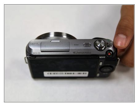
• Turn off the camera by sliding the power switch.
