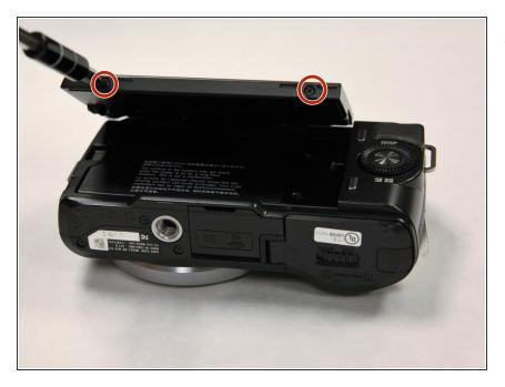
Use a Phillips head 000 screwdriver to remove the two 2.0mm screws on the bottom of the LCD screen.
