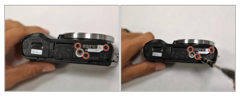
Use a Phillips head 000 screwdriver to remove the three 4.0mm screws on the bottom of the camera.
