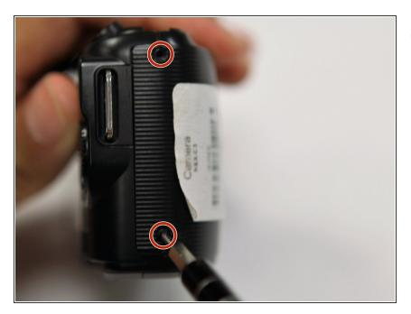
• Use a Phillips head 000 screwdriver to remove the 4.0mm screw at the side opposite of the USB port.
