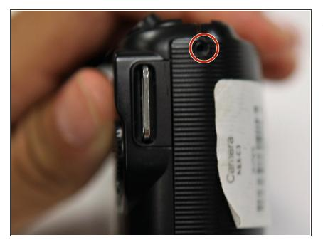
Use a Phillips head 000 screwdriver to remove the one 4.0mm screw on the side opposite of the USB port near the shutter button.
