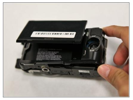
• Gently pry off the back panel, by wiggling it around the LCD screen.
