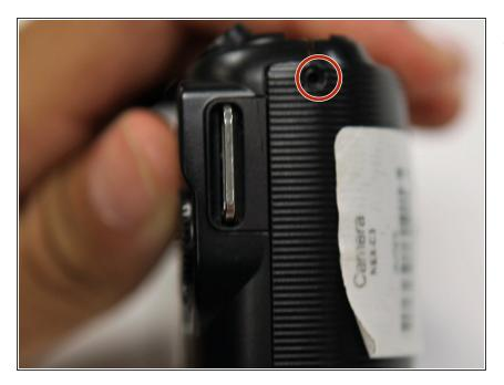
Use a Phillips head 000 screwdriver to remove the one 4.0mm screw on the side opposite of the USB port near the shutter button.
