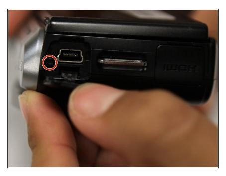
Use a Phillips head 000 screwdriver to remove the 4.0mm screw inside the USB port.
