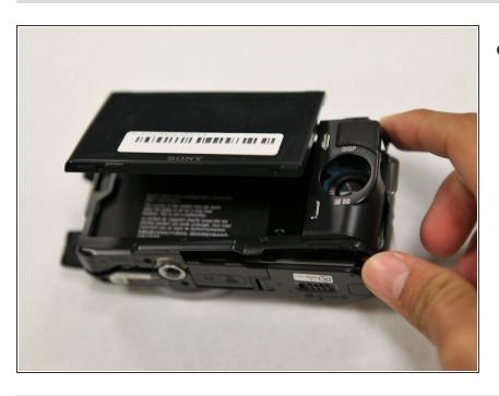
Gently pry off the back panel, by wiggling it around the LCD screen.
