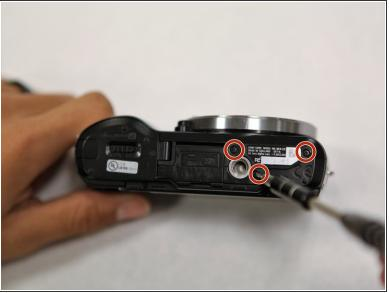
Use a Phillips head 000 screwdriver to remove the three 4.0mm screws on the bottom of the camera.
