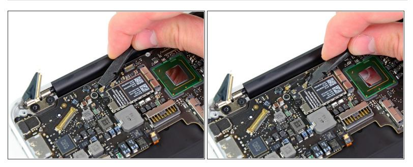
Use the flat end of a spudger to pry both antenna cable connectors up and off their sockets on the AirPort/Bluetooth card.
