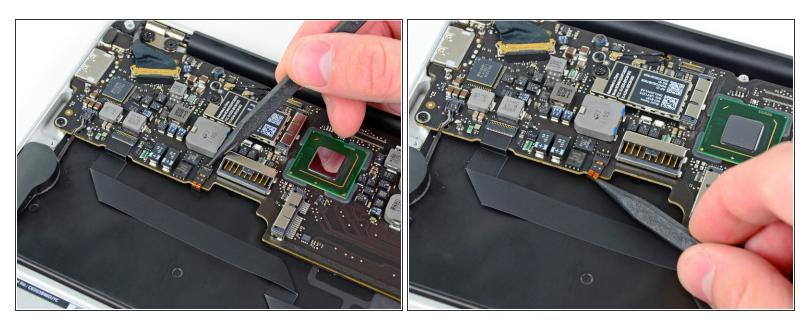
Use the tip of a spudger to flip up the retaining flap on the keyboard backlight ribbon cable ZIF socket.
