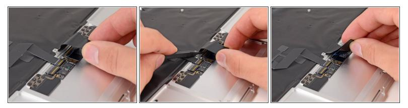
(i) The ZIF connector for the keyboard ribbon cable is hidden under the cable itself.
