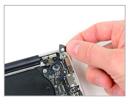
• Remove the small rubber gasket from the corner of the upper case nearest the I/O board.
