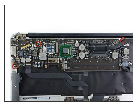
Remove the three 3.6 mm T5 Torx screws securing the logic board to the upper case.
