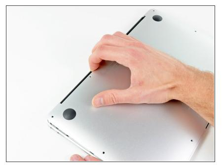
Wedge your fingers between the display and the lower case and pull upward to pop the lower case off the Air.
