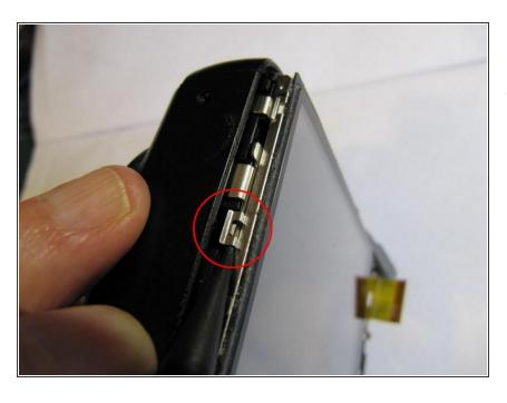
Release a clip on the left hand side of the LCD and hence lift the LCD out.
