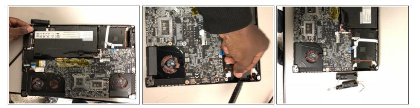
• Disconnect both speaker wires from the motherboard.
