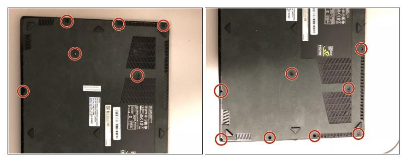
Unscrew the screws located around the bottom panel with a Phillips #00 mm Screwdriver.
