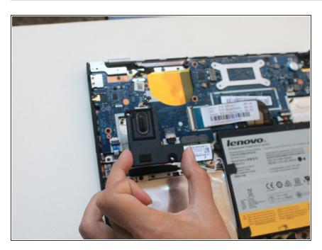
After the cables are disconnected, remove the speakers by lifting the speakers up.
