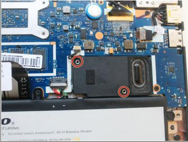
Remove 2 screws (2mm) from each of the speakers, 4 screws total, using the PH #000 screwdriver.
