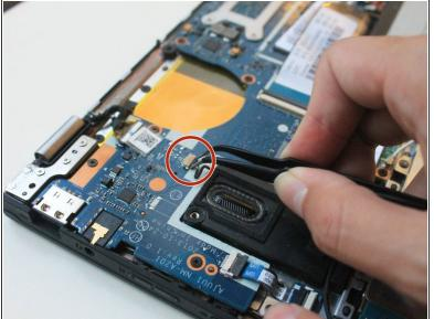
Unclip the cables by pulling downwards gently using tweezers.
