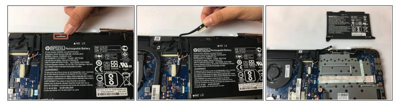
• Carefully disconnect the cable connecting the top of the battery and remove the battery.
