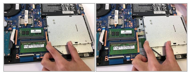
• Disconnect the CD drive from the motherboard connector on the left.
