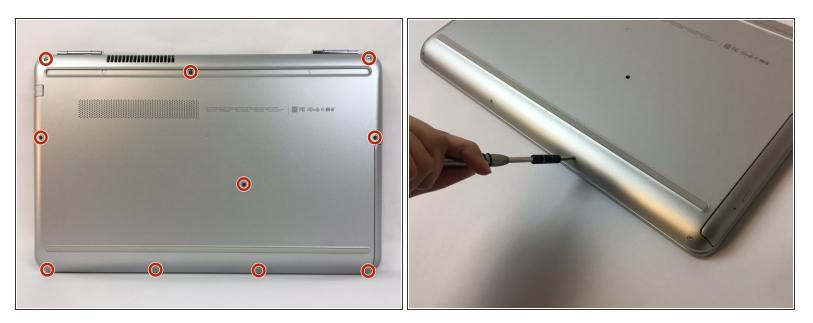
Using a PH0 screwdriver, unscrew the ten 4.4mm Phillips head screws located on the back panel.
