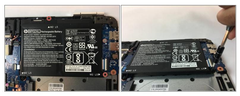
Using a PH0 screwdriver, unscrew the two 3.8mm PH0 Phillips head screws that hold the battery in place.
