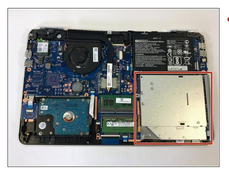
The CD Drive is located at the bottom right area of the motherboard.
