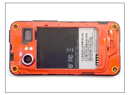
Remove four T6 Torx screws securing the rear inner frame to the front case.
