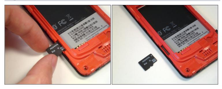
• Pull the MicroSD card straight out of its slot.
