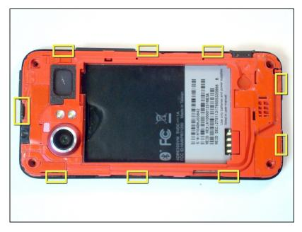
The rear inner frame is attached to the front case by nine plastic clips, marked here for reference.
