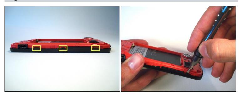
• Rotate the phone 180 degrees and loosen the three clips on the side by the speaker. Note that the middle clip on this side is smaller than the others.
