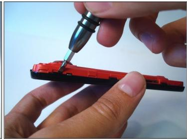
Loosen the clips on the side next to the camera using the method described in the previous step.
