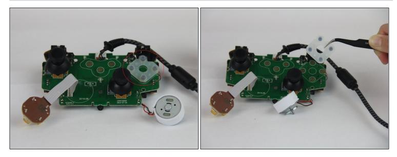
• Go back to the motherboard, and remove the buttons' gasket with a tweezler.
