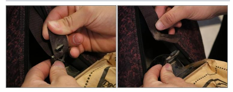
Pull rubber tab attached to recyclable bag off of adjoining plastic tab.
