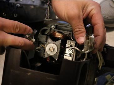
Using the Phillips screwdriver, undo the two screws shown on the front of the black plate and pull out the wires being held within it, carefully.
