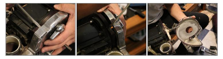
• Use a flat head screwdriver to pry off the front metal plate.
