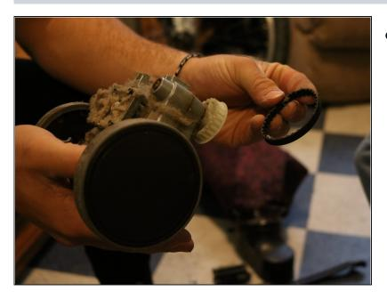
Finish pulling the metal part and attached axles out. If the axels are in need of cleaning, simply clean the existing axels with a wet clothe and put them back into the vacuum. If the axels are in need of replacement, use the new parts you have obtained and place them back in the same place as before and screw them back to the vacuum.
