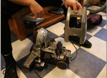
• Remove the metal cover by pulling up, then out.
