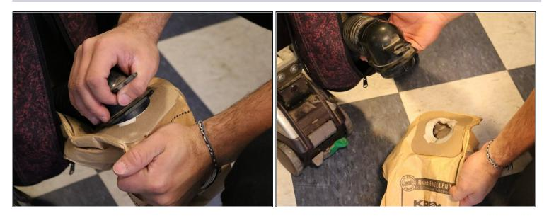
Remove recyclable bag completely by pulling the hose out of the back.
