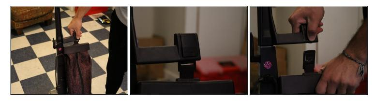
Unclip the top of the dust bag by holding in the clip and pulling down on the bag.
