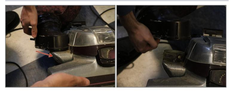
Twist the bottom of the bag counterclockwise and pull to fully remove from the vacuum.
