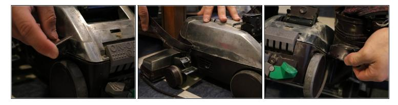
Pull the plastic lining around the bottom of the vacuum off.
