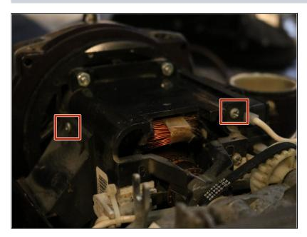
Using a Phillip's head screwdriver, undo the screws on the backside of the vacuum
