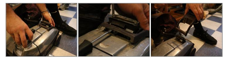
• Remove the plastic covering on the back by using a flat head screw driver to carefully pry up the edges.
