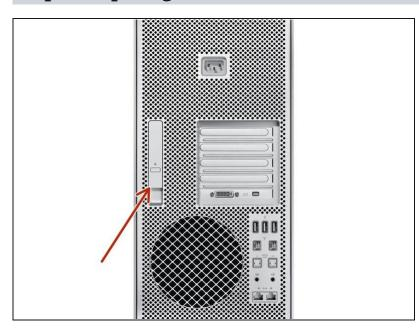
• Then open your Mac Pro by releasing the latch on the back of the machine, it should look like the picture, if you have trouble releasing this latch, use as much force as possible, it takes strength to work on this machine.
