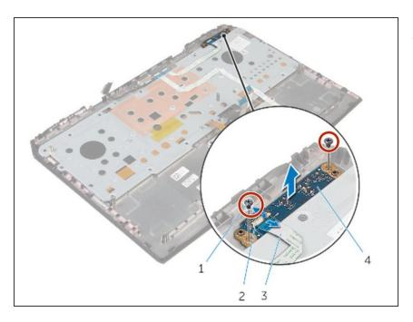
Replace the screws that secure the status-light board to the palm-rest assembly.
