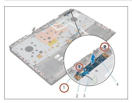
Align the screw holes on the statuslight board with the screw holes on the palm-rest assembly.
