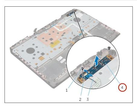
• Slide the status-light board cable into the connector on the status-light board and press down the latch to secure the cable.
