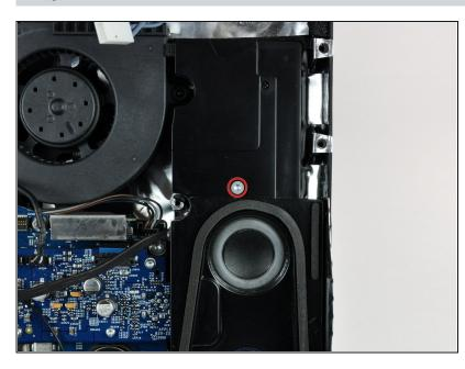
Remove the single 12 mm T10 Torx screw securing the right speaker to the rear case.
