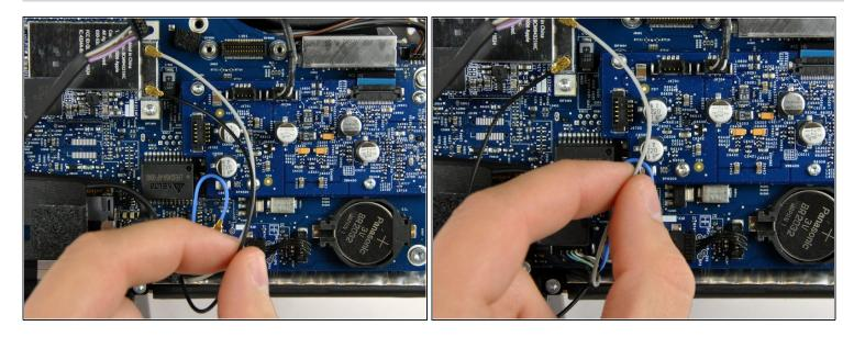
• Move the antenna cables away from the audio board.
