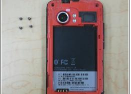
Remove 4 corner screws, you may have to remove a "VOID" sticker from one of the screw heads.
