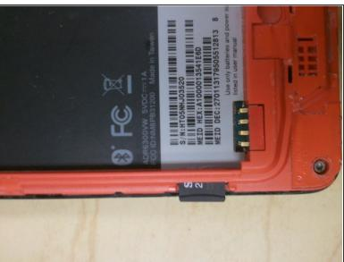
Depress MicroSD to eject it from the side of the case.
