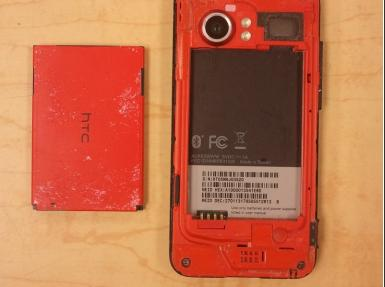
Remove battery, prying from the provided gap at the upper-right corner of the battery
