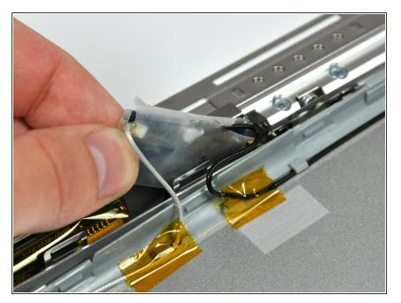
• Lift the antenna board out of the clutch cover.
