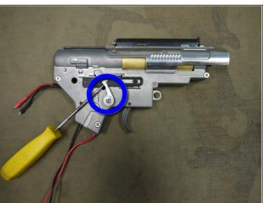
Now remove the the selector link piece by putting a tool underneath long section shown and prying it upward.
