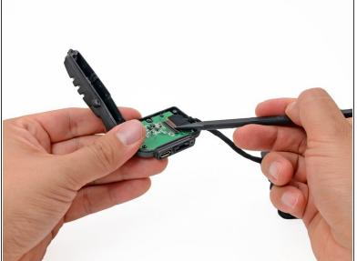
• Use the tip of a spudger to flip up the retaining flap on the button board data cable ZIF connector.
