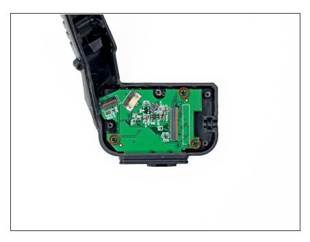
Remove the three 4.5 mm Phillips screws securing the button board to the viewfinder housing.
