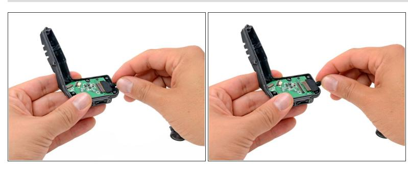
Remove the button board data cable from its socket on the button board.
