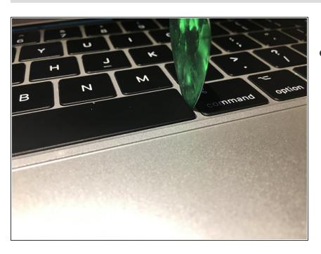
Slide a thin guitar pick or card (not a credit card, most are too thick) vertically down the right edge of the key.
