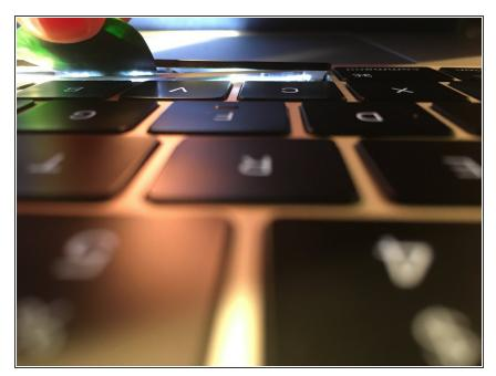
The spacebar on the 2016 MacBook Pro has 3 layers: the top black layer (the keycap), an intermediate white plastic layer (the scissor clip) and the bottom layer (the base of the keyboard). We are going to work our way between the keycap and the scissor clip, as this way the keycap can be removed, cleaned and replaced without damage.
