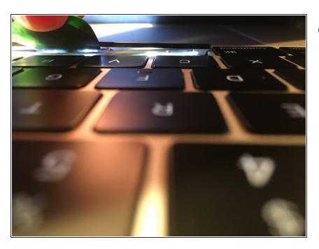
Before you start, <u>READ THE</u> <u>WHOLE GUIDE FIRST</u>. This is fiddly and you especially need to see the bottom of the key before you start (steps 8 and 9). If you aren't careful you will damage your spacebar, and spares are currently difficult or impossible to obtain due to the laptop's newness.
