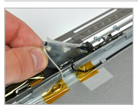
Lift the antenna board out of the clutch cover.
