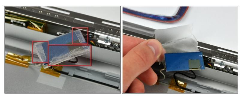
Peel back the three edges of the antenna board cover and remove it from over the antenna board.
