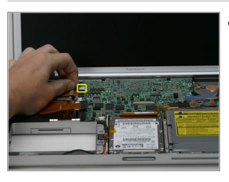
Disconnect the inverter cable from the logic board.
