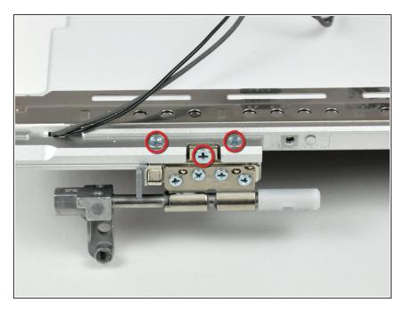
Remove the three Phillips screws securing the right clutch hinge to the front bezel.
