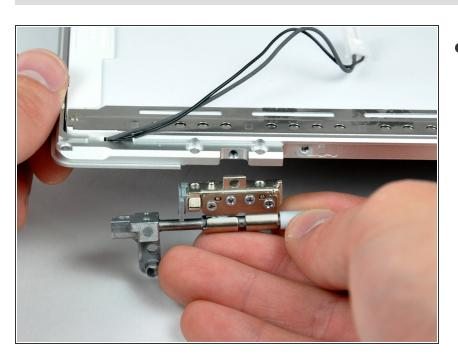
Remove the right clutch hinge from the front bezel.
