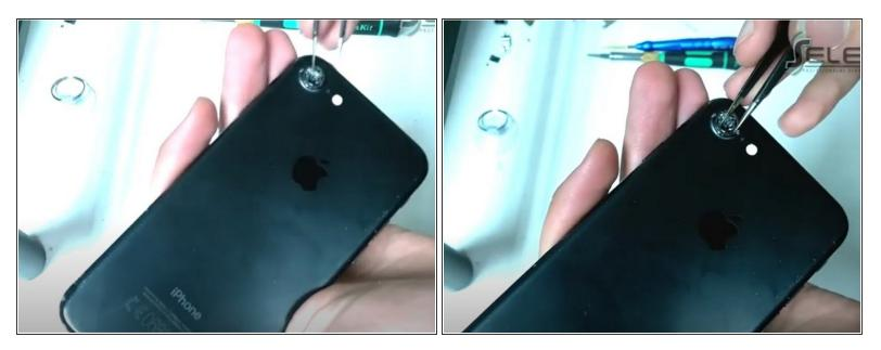
Use a pair of tweezers to carefully remove the remains of any broken glass from the cracked camera cover.
