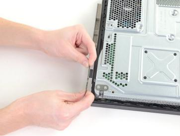
Pull the front circuit board straight out away from the upper metal case and set it aside.
