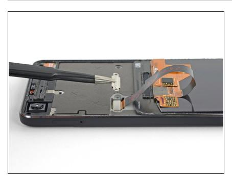
• Remove the display cable bracket.
