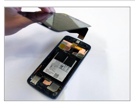
Pull the screen up to fully remove it.
