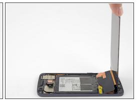
Lift the earpiece end of the display up to provide access to the display cables.
