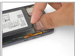
• Using a pair of tweezers or your fingers, grab the black battery pull tab and slowly pull it upwards until the corner is loose.
