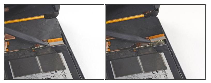
Use the point of the spudger to lift and disconnect the display cable connector from its socket.
