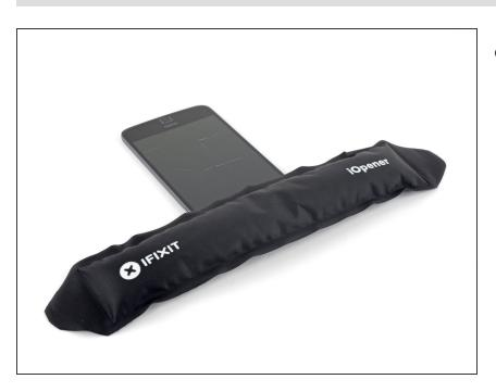
Apply a heated iOpener to the top edge of the phone for at least 90 seconds.
