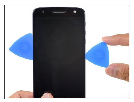
Repeat the heating, lifting, and cutting steps for the remaining long edge of the phone.
