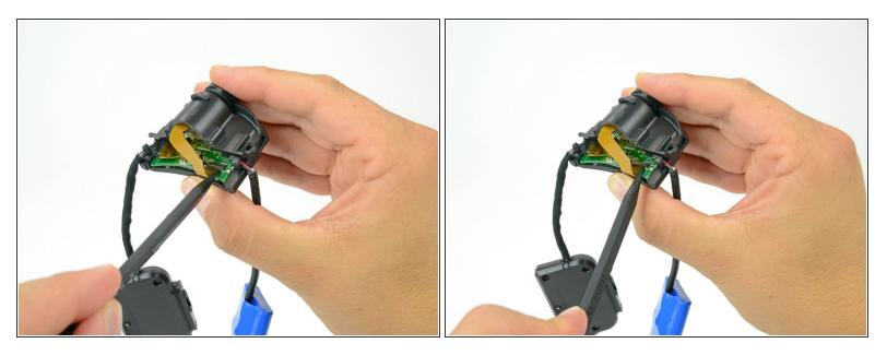
• Use the tip of a spudger to pry up the retaining flap of the camera sensor cable ZIF connector on the motherboard.
