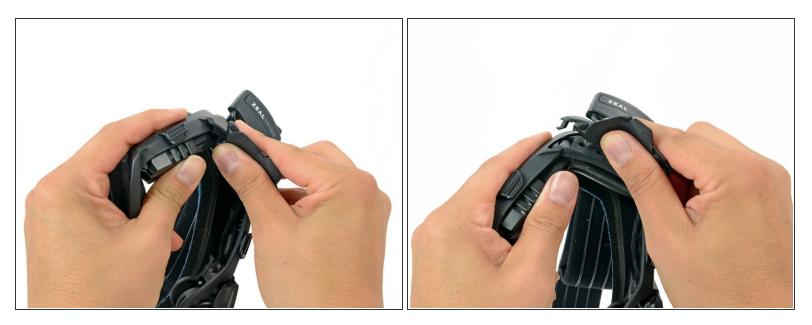
Once the bottom is free, continue pulling to free the bottom of the strap mount cover from the frame.
