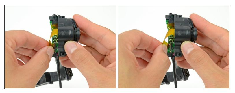
• Pull the camera sensor ribbon cable straight out of its connector on the motherboard.
