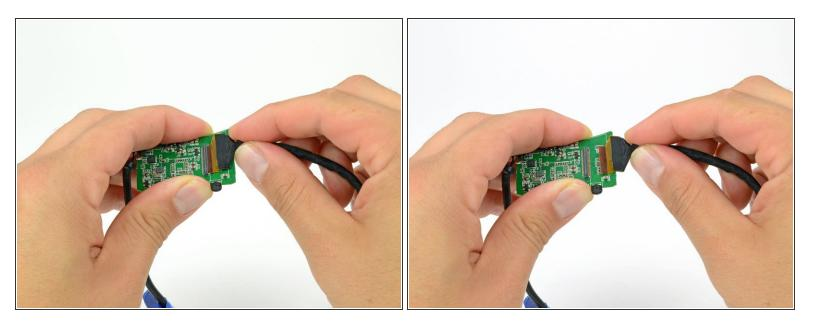
• Pull the viewfinder assembly ribbon cable straight out of its socket on the motherboard.
