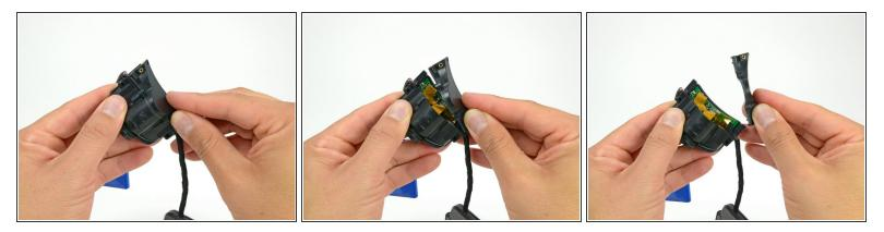
• Lift the back cover off the camera housing and remove it.
