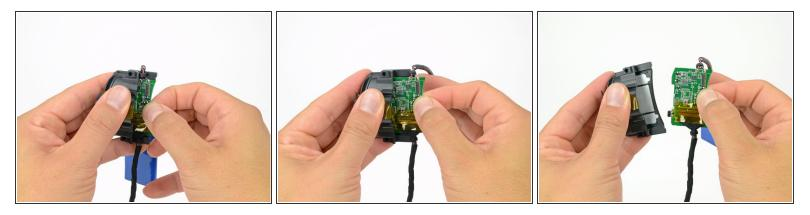
• Grab the edge of the motherboard and gently slide it out of the camera housing.
