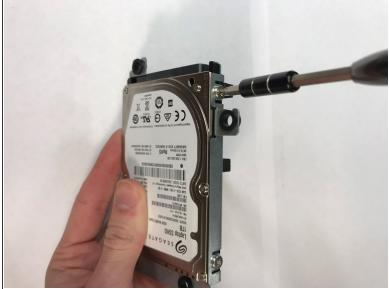
• Unscrew the four screws that hold hard drive enclosure to the hard drive, located on the side of the enclosure.
