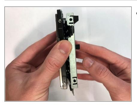
• Lift the hard drive up to remove it from the enclosure.
