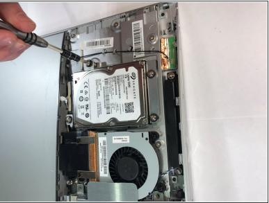
Unscrew the four screws that secure the hard drive enclosure.
