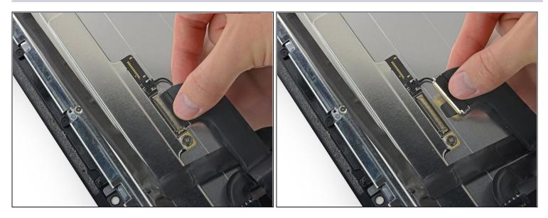
• Pull the display data cable connector straight out of its socket on the back of the display.
