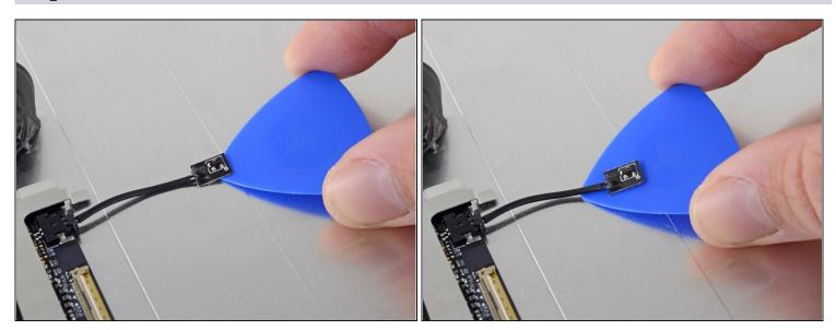
• Use an opening pick to break up the adhesive holding the thermal sensor to the back of the iMac display.
