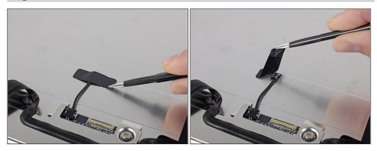
Peel up the piece of tape securing the thermal sensor to the back of the display assembly.
