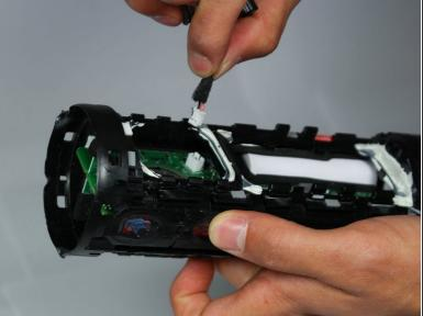
• Once speaker is detached from casing, remove cable from motherboard.
