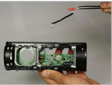
With the ribbon cable disconnected from the motherboard, remove the Bluetooth antennas.
