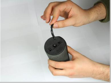
Remove the rubber port cover, peeling up from one end.
