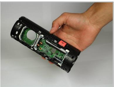
With both the speaker and passive radiator removed from one side of the Boom 2, repeat steps 13-18 for the other side.
