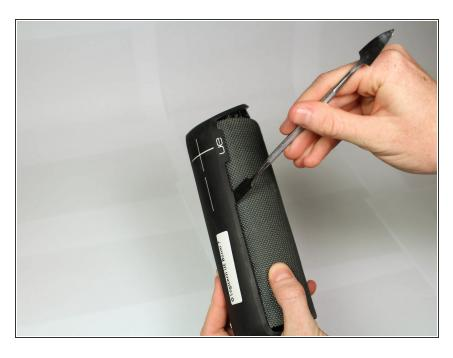
Continue removing the rubber stripping down the side.
