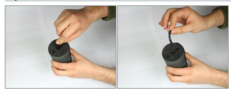
• After the D-ring has been removed, remove the rubber port cover.
