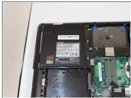
Remove the optical drive from the device.
