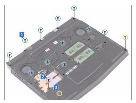
Remove the (M2x3) screw that secures the computer base to the palm-rest assembly.
