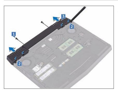
Using a plastic scribe, gently release the tabs that secure rear-I/O cover to the computer base.
