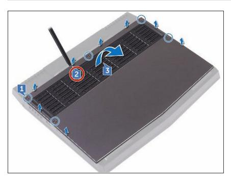
Using a plastic scribe, gently pry the base cover to release the tabs on the base cover from the slots on the computer base.
