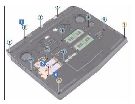
Align the screw holes on the NEW computer base with the screw holes on the palm-rest assembly.
