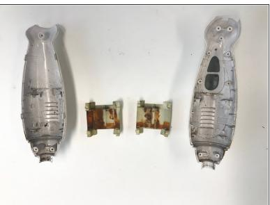
To disassemble the motor holders you can slide them of the casing.
