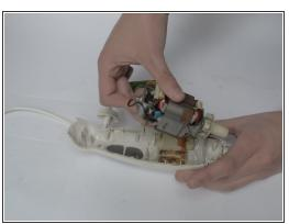
Unscrew 4 screws to disassemble the printplate and 2 to unscrew the wiring. Then you can lift the motor out by hand.
