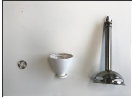
To disassemble the 3 parts you've got to disconnect the little ring. Use a screw driver to get the ring loose.
