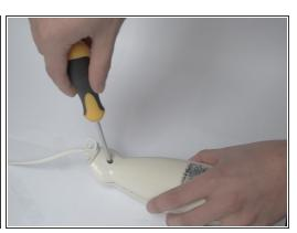
Unscrew 3 screws to open the casing.
