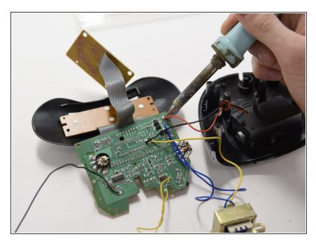
• Remove all the electrical components by desoldering.
