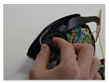
• Remove the gear that protects the cap.
