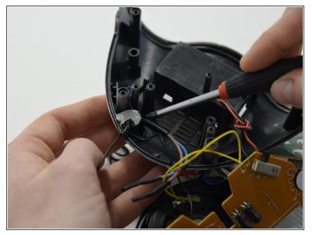
• Remove the hot glue of the antenna.
