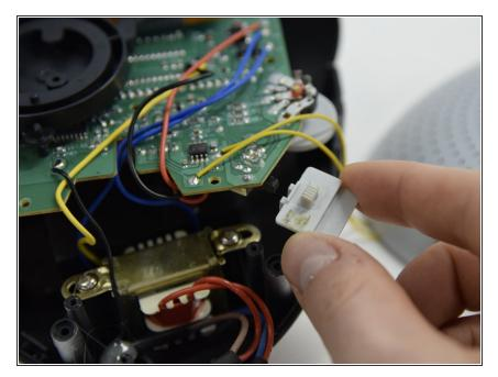
• Remove the switch casing.
