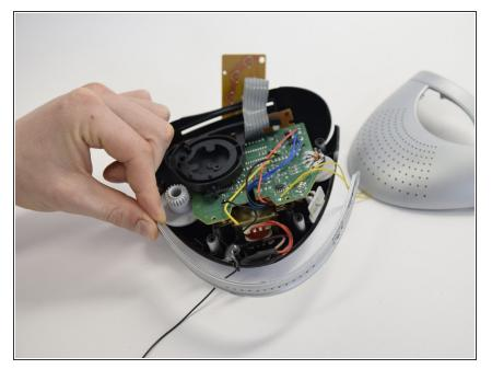
• Remove the backside of the casing.
