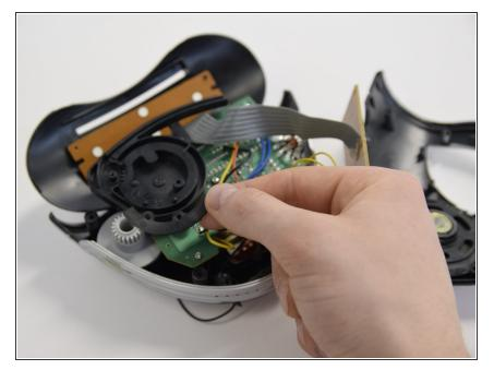
• Remove the flexible pin rack holder.
