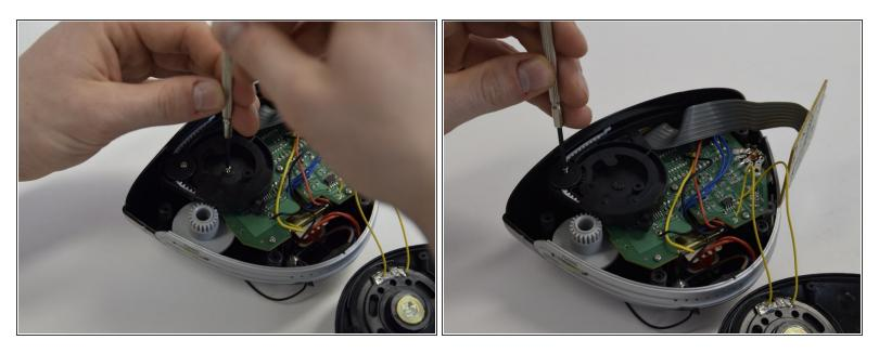
• Unscrew 2 screws of the radio tuning system.
