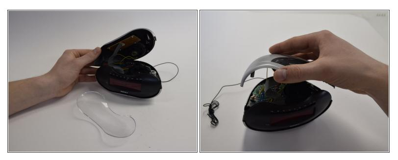
• Open the top and remove the transparent plastic cap.
