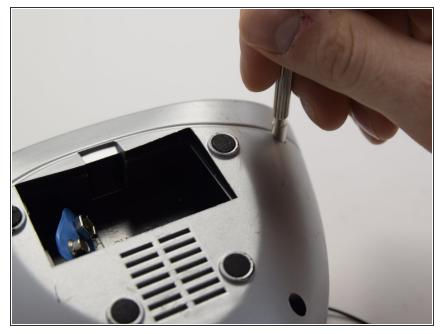
Unscrew the 4 base screws at the bottom with the Phillips 1 screwdriver.
