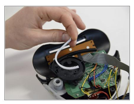
• Lift up the flexible pin rack.
