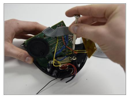
Unscrew 2 screws of the electro magnet.
