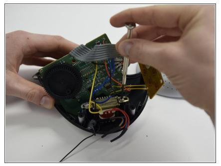
• Unscrew 2 screws on the back of the PCB the black gear house.
