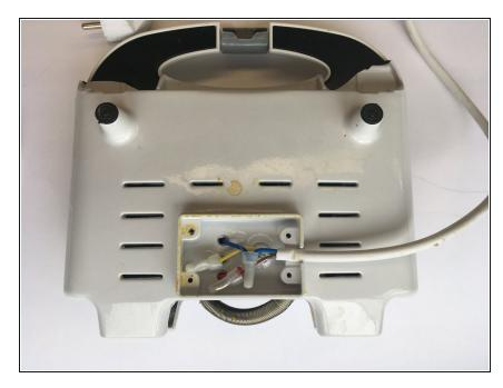
Remove screws from cable housing and remove housing.
