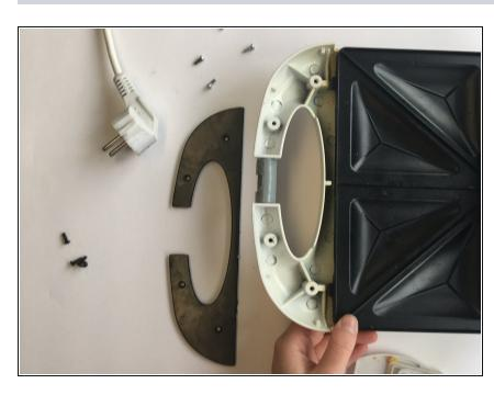
Remove screws from aesthetic handle cover and remove cover.
