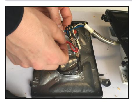
Unscrew and remove the cable harness.
