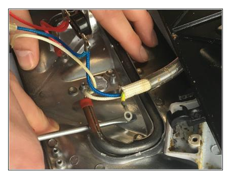
Unscrew and remove the heat sensor.
