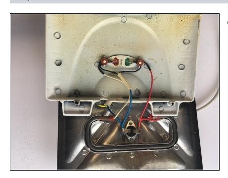
• Remove red rubber insulation rings.
