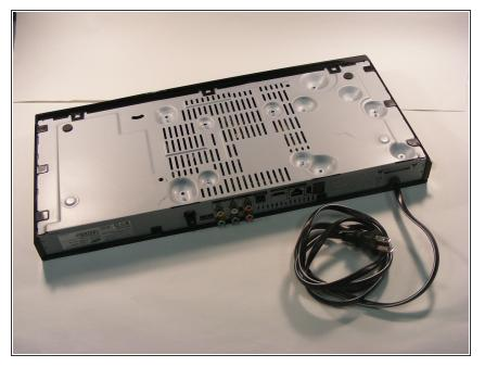
• To begin, turn the device over so that the bottom is facing up. There are 9 black clips that attach the plastic body to the case. Remove these clips from the case.
