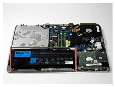
The battery is on the bottom left side.
