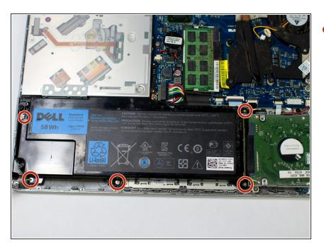
Unscrew the five 4.5mm Phillips #0 screws around the battery.
