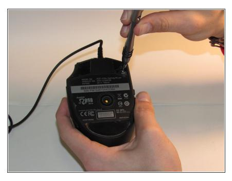
Remove the four 7mm screws using a Phillips #00 screwdriver.
