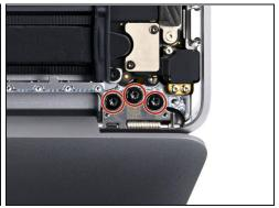
Support the screen with one hand and use your free hand to remove the six T8 Torx screws securing the hinges.
