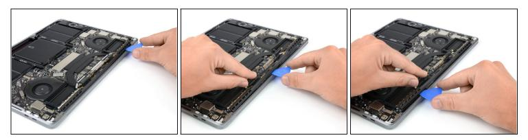
• Use an opening pick to lever out the antenna cable assembly in the areas shown.
