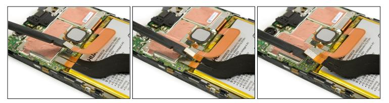
Use the flat end of a spudger to disconnect the three flex cables.
