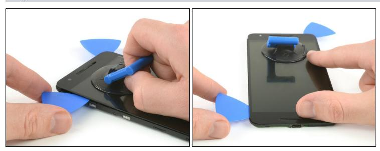
• Slide the opening pick from the top left corner down the left side of the smartphone to the bottom left corner.
