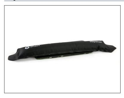
• <u>Use an iOpener</u> to loosen the adhesive under the display.
