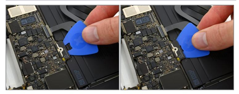
As an added precaution, you may physically disconnect the battery by inserting a <u>battery</u> <u>isolation pick</u> between the logic board and the battery connector.
