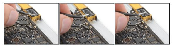
Pry up the second antenna connector to disconnect it.
