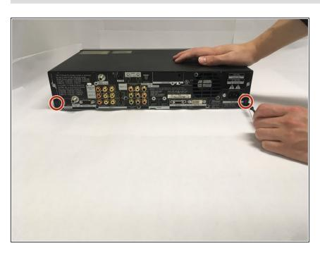
Remove the two 6.5 mm Phillips screws on the back of the device casing.
