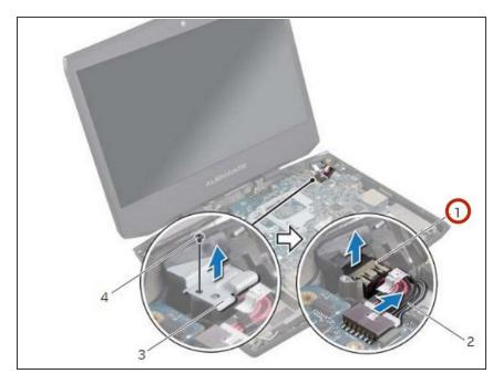
• Lift the power-adapter port off the computer base.
