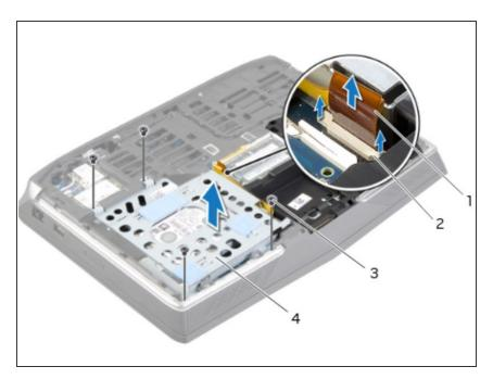
• Turn the secondary hard-drive assembly over.
