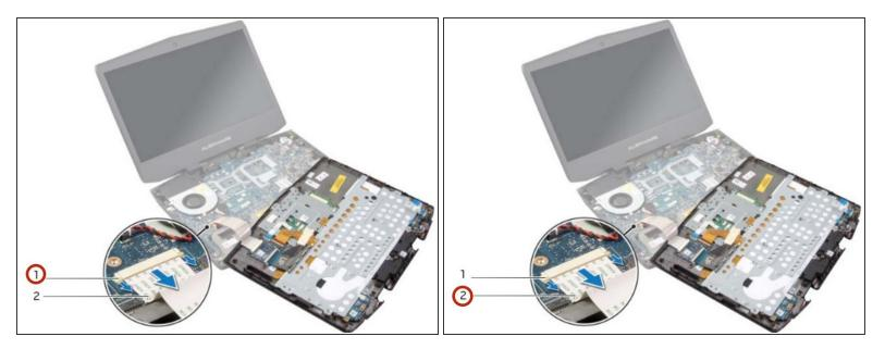
• Release the connector latches to disconnect the flexi-cable from the system board.
