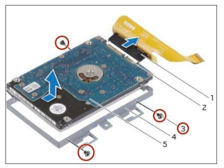
Remove the screws that secure the secondary hard-drive to the secondary hard-drive bracket.
