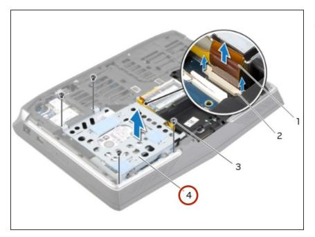
• Lift the secondary hard-drive assembly off the computer base.
