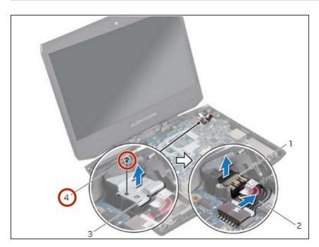
Remove the screw that secures the power-adapter port bracket to the computer base.
