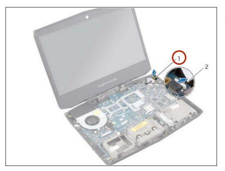
• Disconnect the tron light from the optical fibre.
