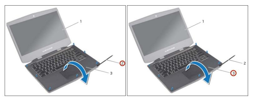
• Using a plastic scribe, pry the palm-rest assembly from the computer base.
