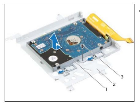
Turn the secondary hard-drive assembly over.
