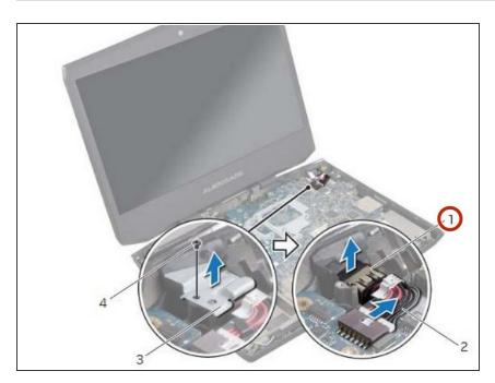
• Align the **NEW** power-adapter port with the slot on the computer base and slide the power-adapter port into place.
