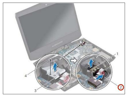
Connect the power-adapter port cable to the system-board connector.
