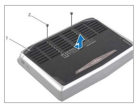
Align the tabs on the NEW base cover with the slots on the computer base and slide the base cover into place.
