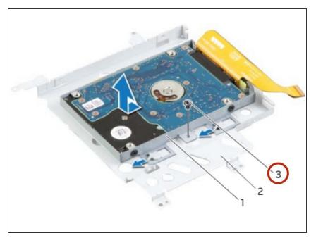
• Remove the screw that secures the secondary hard-drive assembly to the main bracket.
