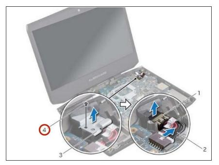
Replace the screw that secures the power-adapter port bracket to the computer base.
