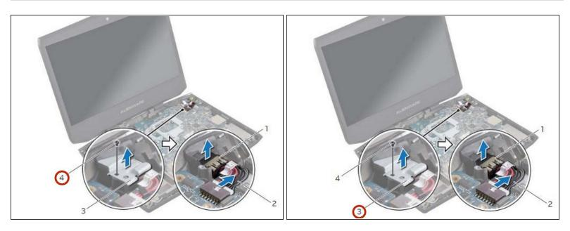
• Align the screw hole on the power-adapter port bracket with the screw hole on the computer base.
