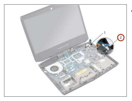
• Connect the tron-light cable to the system-board connector.
