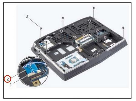
Slide the status-light board cable into the system-board connector and press on the connector latch to secure the cable.
