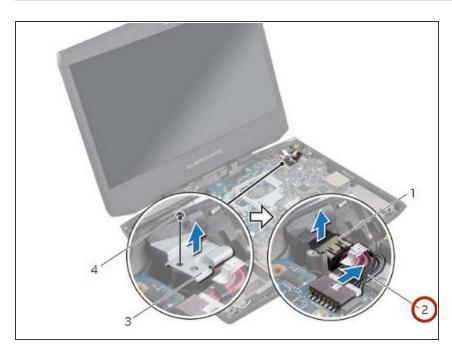
• Disconnect the power-adapter port cable from the system-board connector.
