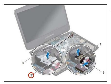
• Lift the power-adapter port bracket and keep it aside.
