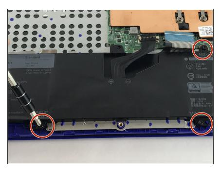
With the J1 screwdriver bit, unscrew three (3) size 40 mm battery screws.
