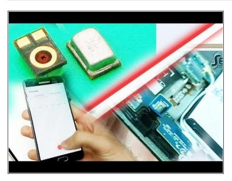
Soldering new microphone to the SAMSUNG GALAXY A5 2016 mainboard.
